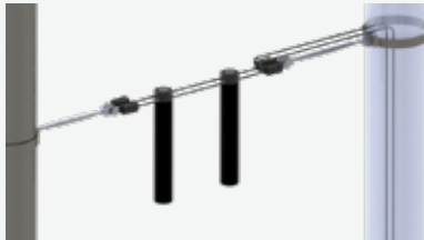
Poles and tree mounting set for diameters 50 - 441mm
