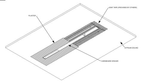
DO NOT PLASTER OVER THE OPENING OF THE HOUSING OR THE LOW VOLTAGE WIRE.
